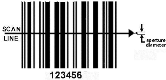
Figure 1 - Scan Line through a Bar Code
