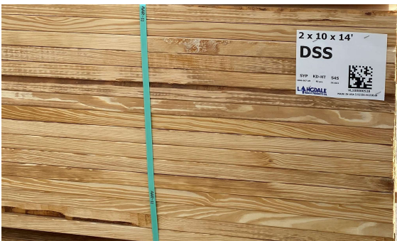
2D Datamatrix Bar Code on Pack of Finished Wood Products
